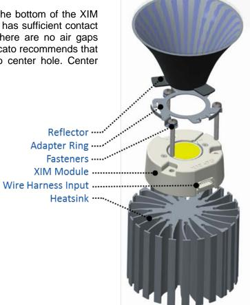
Figure 2: XIM Assembly (Exploded View)
