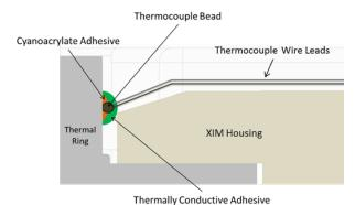
Figure 7: Cross-section of Xicato recommended thermocouple attachment.
